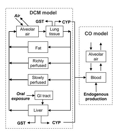
Figure C-1. Schematic of the PBPK model for dichloromethane in the rat.
